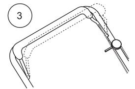
3. Hold the mower's brake handle closed.
